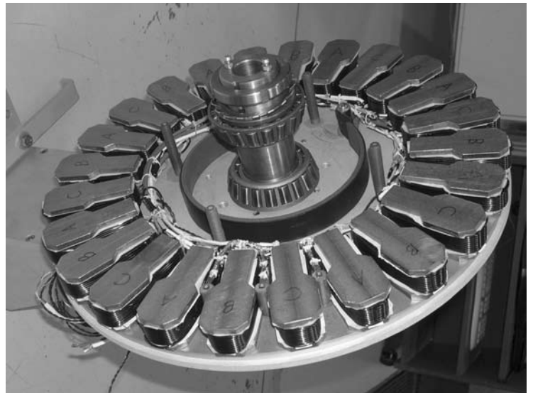
Internal coil arrangement, bearing and spindle assembly
