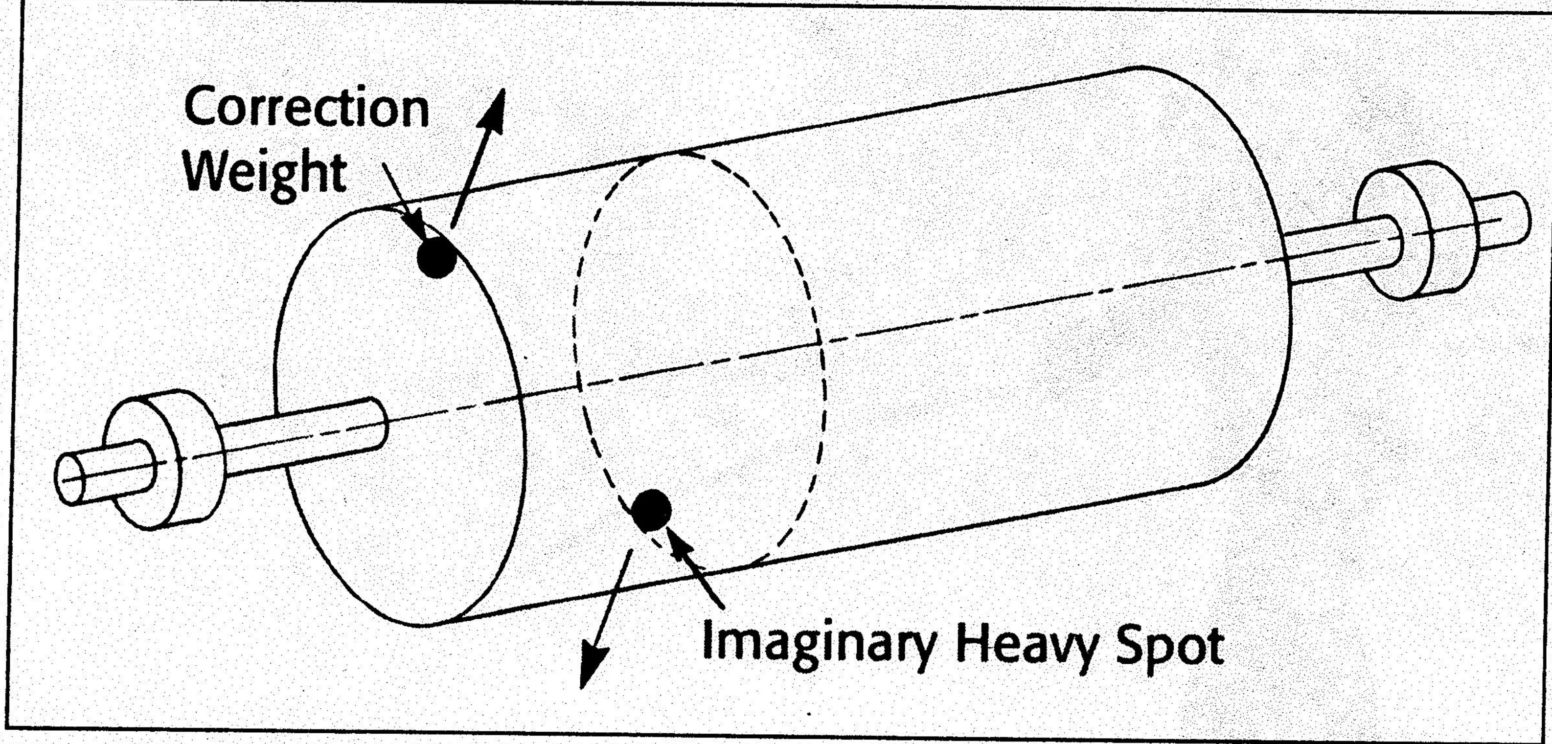
Figure 1: The correction weight plane is offset from the heavy spot plane, creating a couple unbalance condition.
