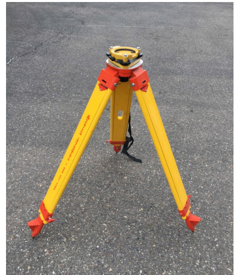
Figure 21: Tripod 3-point support for stability.
