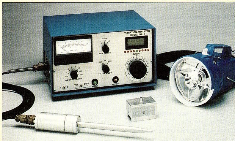
Field balancing instruments include tunable filter type. (Photographs courtesy Balmac, Inc. [top] and Diagnostic Instruments, Inc. [bottom].)
