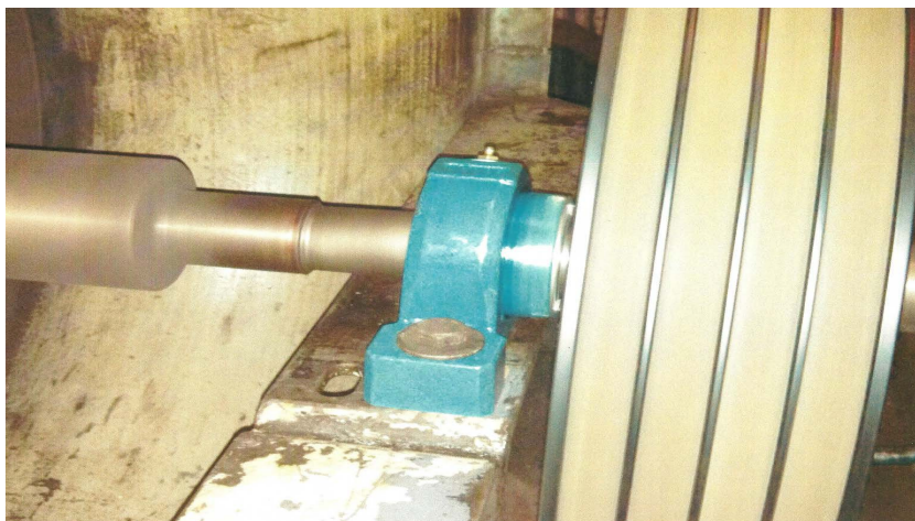
Figure 5. New Bearing Installed to Right of Grooved Shaft
